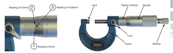
To get to the final reading size of a micrometer above we add up the three readings
